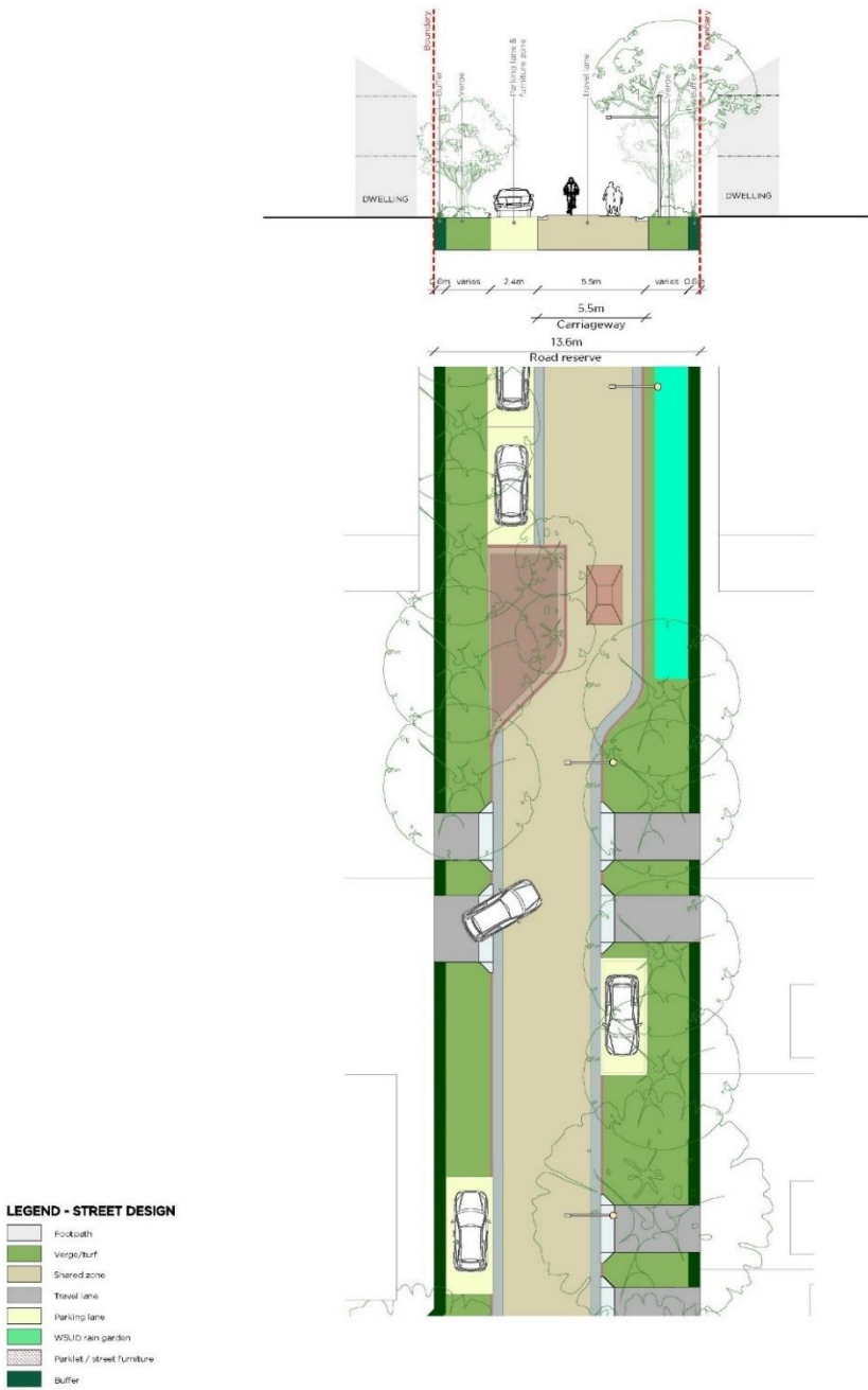
Figure 52: Shared Zone C1 - section and plan
